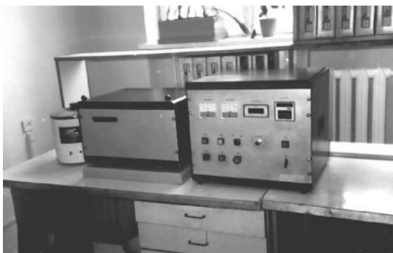
Fig. 1 A device for determining the dynamic strength of diamond powders such as Fraitester
