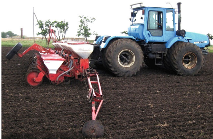
Fig. 1 Seeding aggregate including HTZ-170 tractor and “Kverneland Optima” seeder
